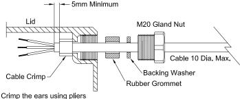
so the ring is as tight as possible on the cable outer sheathing.
